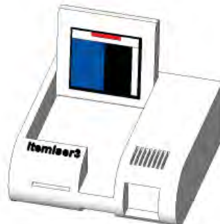
GE IonTrack Itemiser 3 Isometric View
